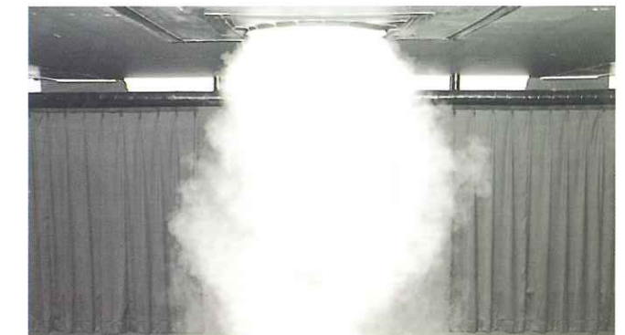
Vertical air supply in heating
