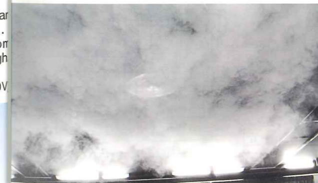
Horizontal air supply in cooling
